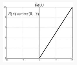
Activation function that allows neural network to capture nonlinearity
