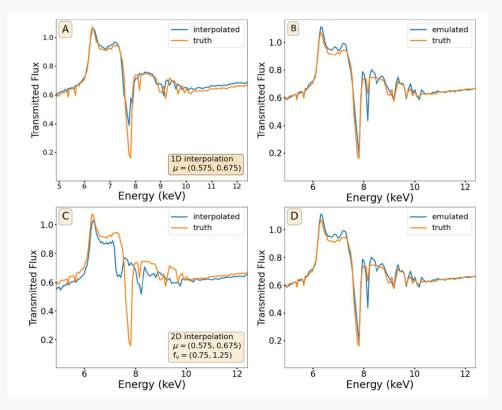
Comparison between linear interpolation and interpolation performed by a neural network
